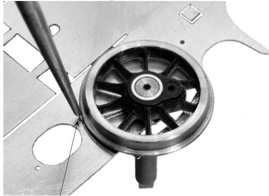
Then using a wheelset with a turned bearing on the axle. Scribe around the wheel edge
