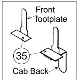
19. Check positioning and fit cab interior castings.
