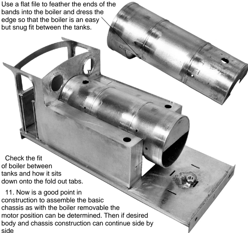
Check the fit of boiler between tanks and how it sits down onto the fold out tabs.
