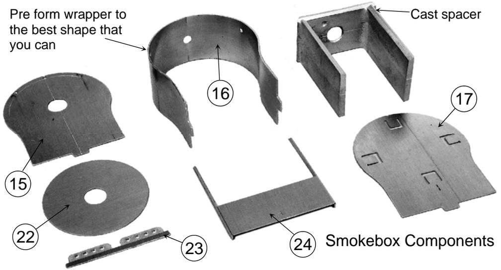
9. Secure the smoke box front (part 15) to a block of wood using drawing pins and solder the wrapper (part 16) around the edges so that the front acts as a former. Start by positioning the wrapper to the centre of the smoke box front top, there being a small half etched centre line mark to aid positioning.
