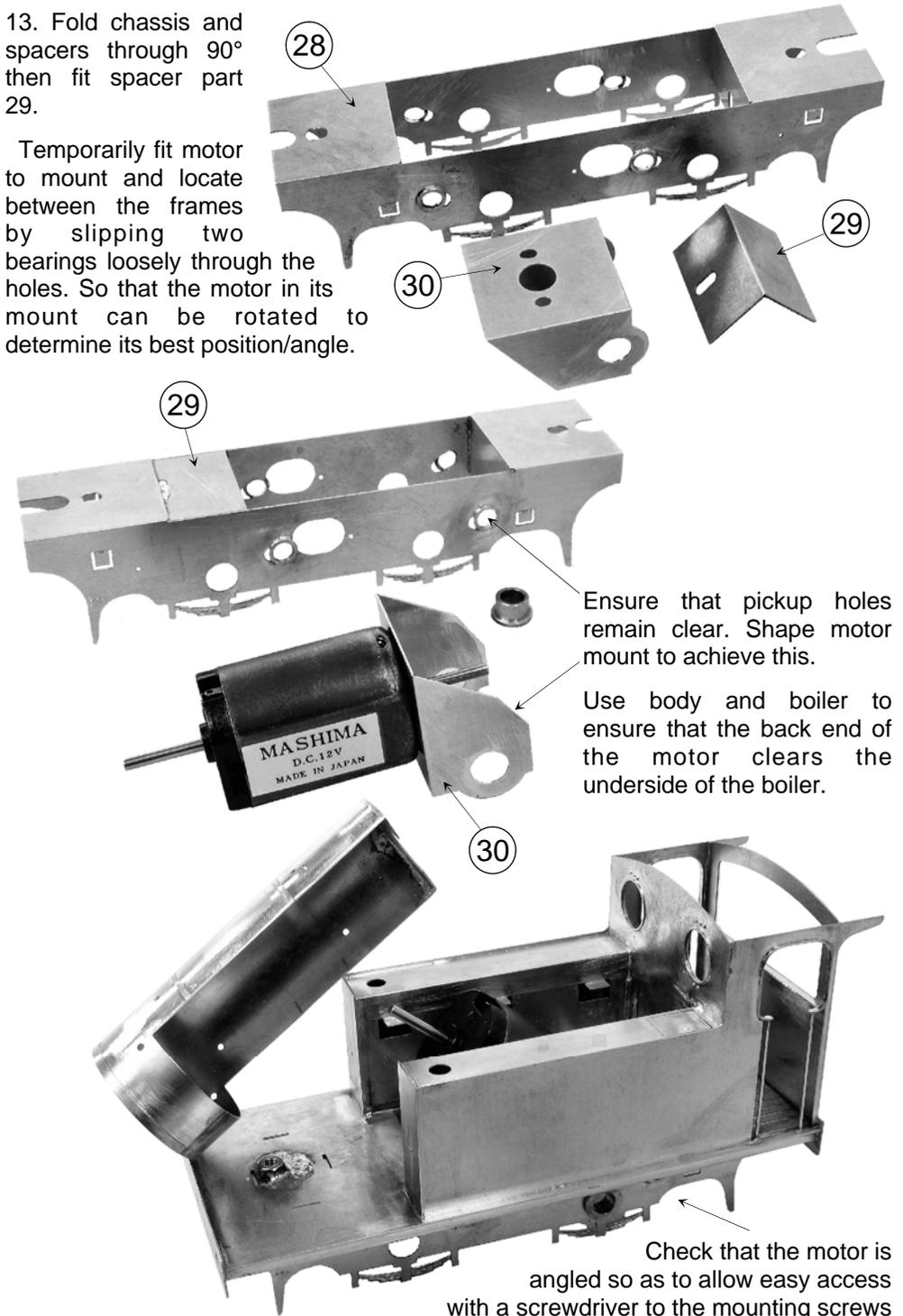
Ensure that pickup holes remain clear. Shape motor mount to achieve this.
