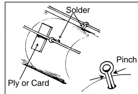
I close up the eye of the split pin to be a loose fit around the wire before fitting into the hole in the boiler and use a piece of card to space the handrail evenly away from the boiler. For the curved smoke box front handrail I find it helpful to anneal the wire in a cigarette lighter flame and then form about twice the length needed to the required radius. This extra length will be easier to handle when spacing away from the smoke box and you can trim to length after soldering solid.
