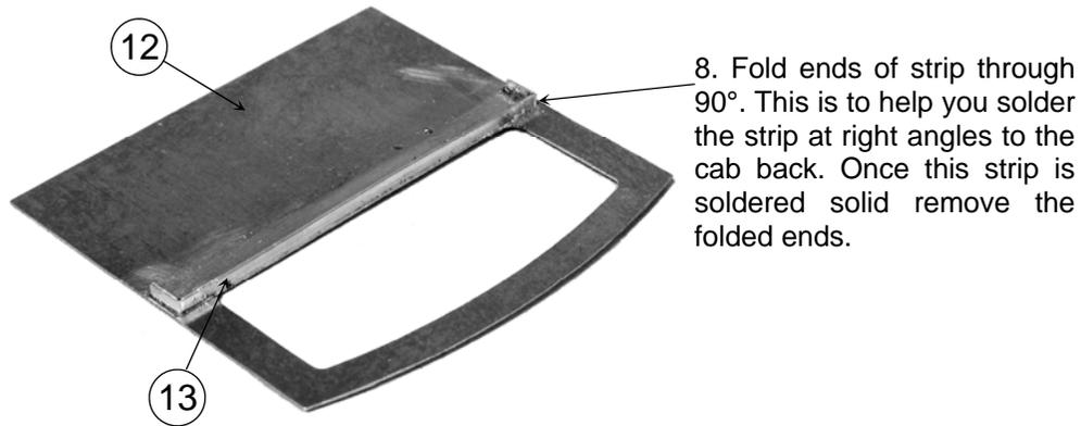
8. Fold ends of strip through 90°. This is to help you solder the strip at right angles to the cab back. Once this strip is soldered solid remove the folded ends.
