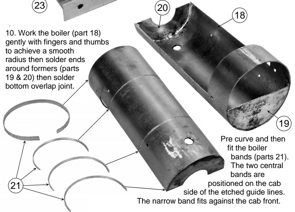
Pre curve and then fit the boiler bands (parts 21). The two central bands are positioned on the cab side of the etched guide lines. The narrow band fits against the cab front.
