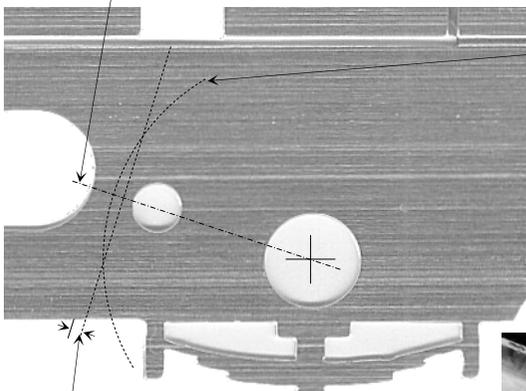
Then scribe a line through what will be the new pickup centre point (just over 0.5mm from the wheel edge).
