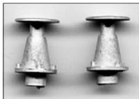
Originally a bell shaped whistle was fitted onto the cab roof but photos show many locos running with an organ pipe type.
