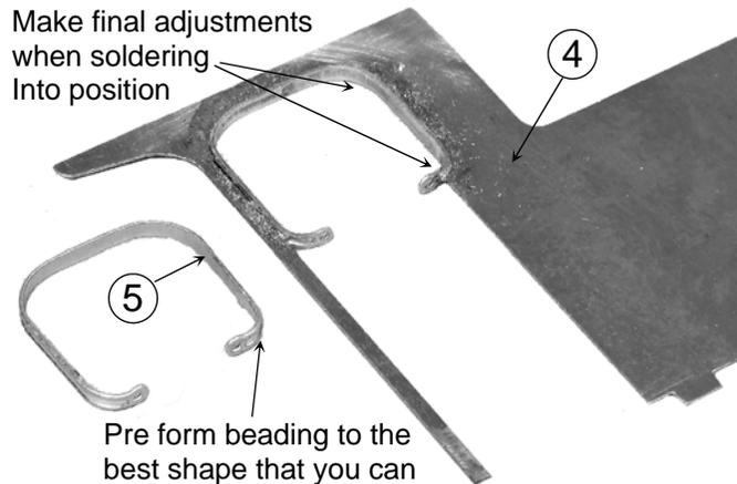
Make final adjustments when soldering into position
