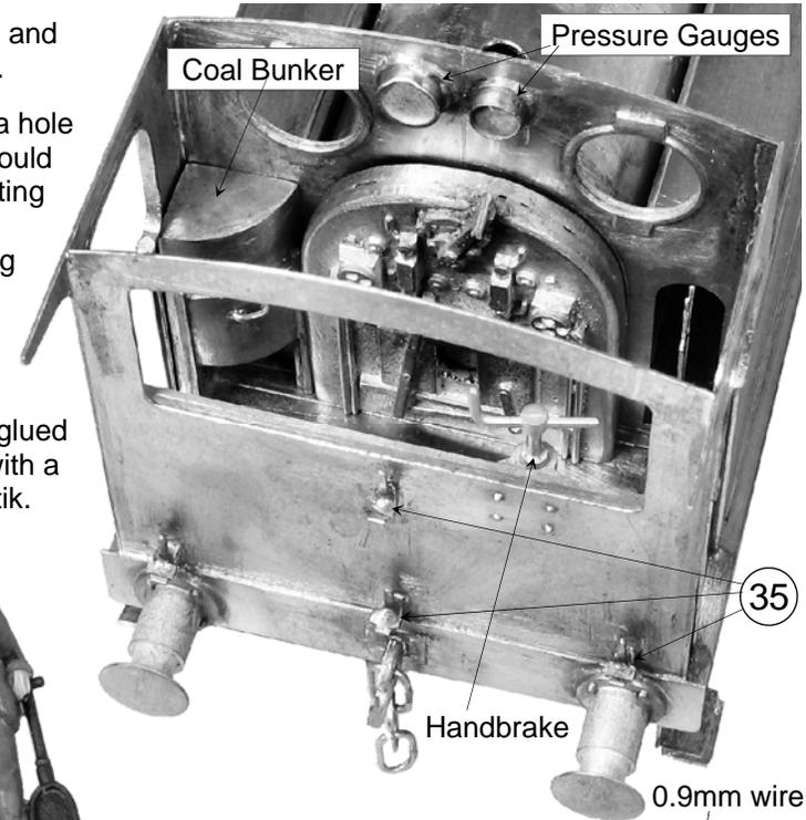
Two part backhead. I would recommend painting separately and then fitting into the painted loco by passing through the cab back cutout. Glue with Evo-Stik.
