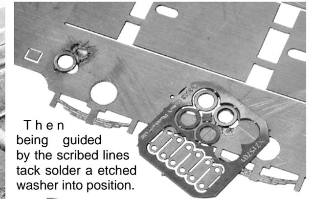
Then being guided by the scribed lines tack solder a etched washer into position.
