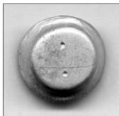
The five post 1923 built locos were fitted with Ross Pop valves mounted on a base. Some changes happened to individual locos during the life of the class caused by boiler swaps etc, so check your photos. I suggest low melt soldering the base casting to the boiler and then drilling at the dimpled positions holes that the valves are a snug (with a spot of Araldite) push fit into.
