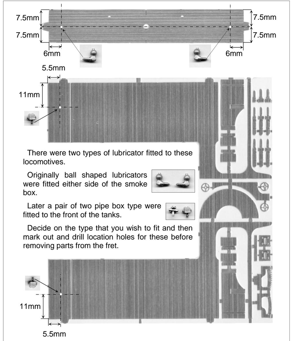
There were two types of lubricator fitted to these locomotives.
