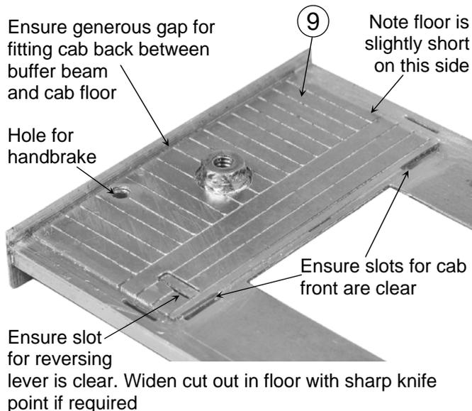
Ensure generous gap for fitting cab back between buffer beam and cab floor
