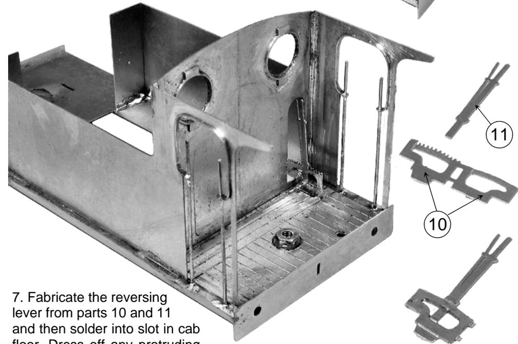
7. Fabricate the reversing lever from parts 10 and 11 and then solder into slot in cab floor. Dress off any protruding tabs on underside of floor.
