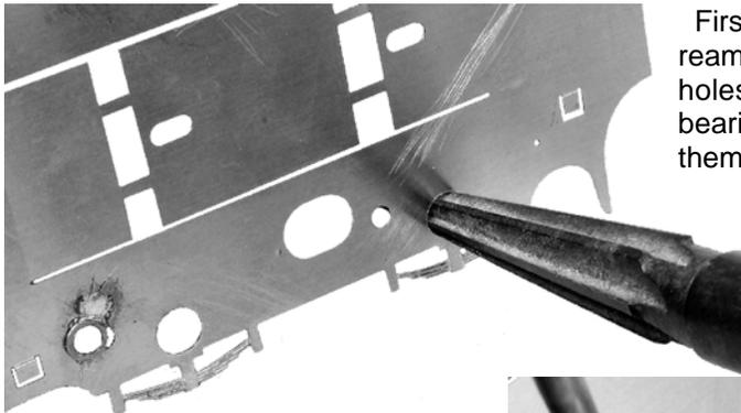
First using your large tapered reamer gently open out the axle holes so that the turned bearings are a good snug fit into them.
