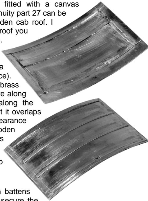
Also fit a strip at the point that the cab back joins the roof.
