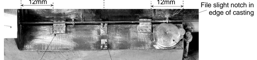
Tank brackets. Original fitting on all locos. File end at angle to blend into boiler curve and get joint between the two L shaped brackets to line up with tank inner edge.
