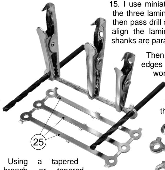
15. I use miniature electrical crocodile clips to hold the three laminates of the coupling rods together. I then pass drill shanks through the crankpin holes to align the laminates. Check by eye that the drill shanks are parallel and square to the rod.
