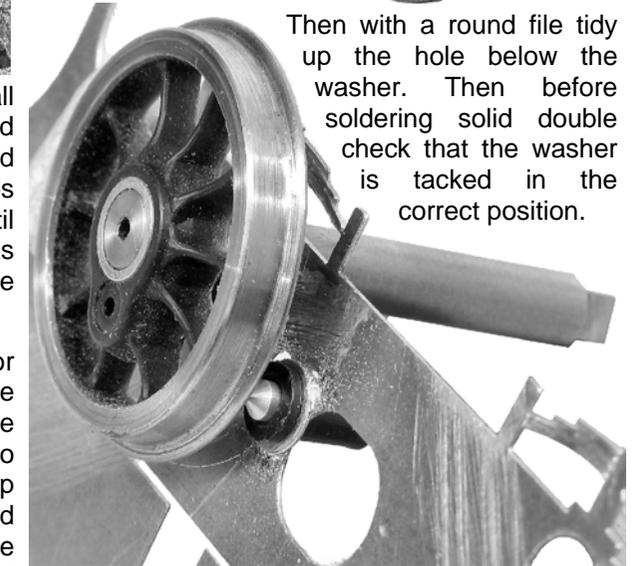
Then with a round file tidy up the hole below the washer. Then before soldering solid double check that the washer is tacked in the correct position.
