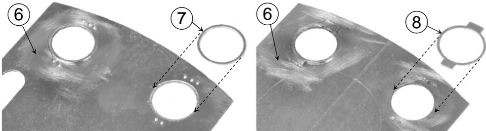
4. Emboss the bolt heads from the rear face and then fit the spectacle rings (parts 7) into the rebates in the cab front (part 6) Then solder the inner spectacle rings (parts 8) onto the rear face so that they cover the bolt holes.
