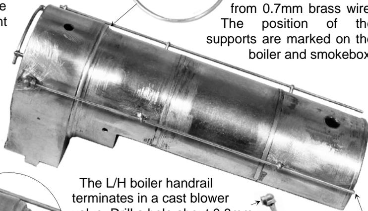
The L/H boiler handrail terminates in a cast blower valve. Drill a hole about 0.8mm diameter into casting to provide a firm fixing for the handrail wire before fitting the casting. Cut rear of handrails flush with boiler end to fit against cab front.
