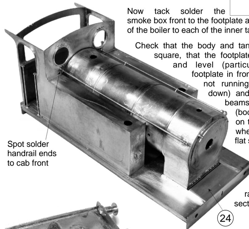
Spot solder handrail ends to cab front
