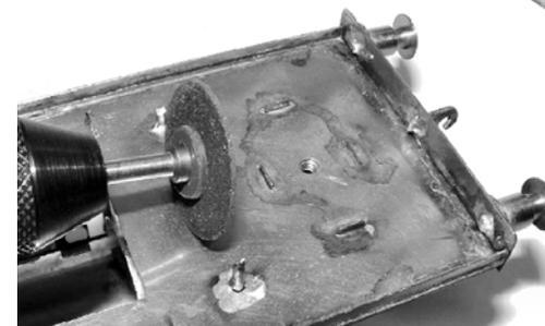
As construction progresses I would recommend trimming any projecting tabs flush so that the body will still sit flat on a block of wood. A grinding disc in your minidrill is ideal for this operation.
