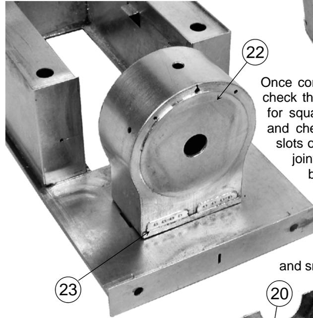
Once completed check the assembly for square (particularly at the bottom) and check that it will fit into the four slots on the footplate. Then dress the joints to blend into the front and back face and form a slight radius to the edge. Any slight creases in the wrapper can be smoothed out using a flat file. Then fit the cylinder end detail overlay (part 23) and smoke box door ring (part 22).
